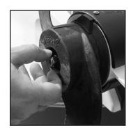
**11.** Re-fasten the propeller onto the armature shaft according to the manufacturer's guidelines.
