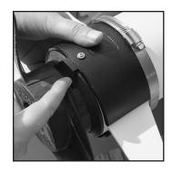
**10.** Make sure the Prop Buddy blades are flush against the rear of the propeller and do not interfere with propeller rotation.
