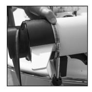
12. Position the hose clamp screwcage behind the skeg and tighten the clamp with a screwdriver. Take care not to overtighten the clamp, as this could damage the composite material.
