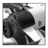
**8.** Completely open the hose clamp and wrap it around the groove in the leading edge of the Prop Buddy collar.
