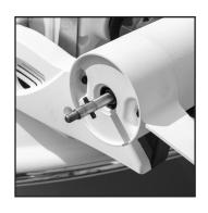
for the first time, take the opportunity to inspect the armature shaft for corrosion and impacted vegetation and perform maintenance according to the manufacturer's guidelines.
