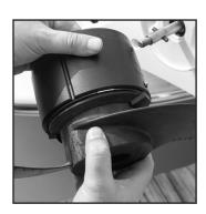
**6.** Insert the motor facing side of the propeller into the bladed side of the Prop Buddy collar.
