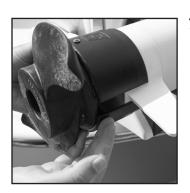
1. Slip Prop Buddy onto the motor housing until the propeller is fully seated on the armature shaft. The opening in the Prop Buddy collar is to accommodate the trolling motor skeg.
