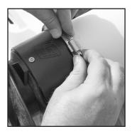
**9.** Insert the loose end of the hose clamp into the screw cage and finger tighten only.
