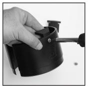
3. Insert one of the provided screws into the screw boss and tighten with a screwdriver. Repeat steps 1-3 with the other blade.
