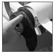
**4.** Remove the propeller according to your trolling motor manufacturer's guidelines.
