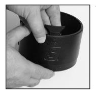
1. Insert one of the blades into the slot on the inside of the Prop Buddy collar (the blade fits only one way). Make sure the screw boss on the blade is inserted into the hole in the collar.
