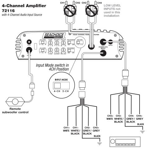
To FRONT and REAR L/R Speaker Terminals of head unit or signal processor
