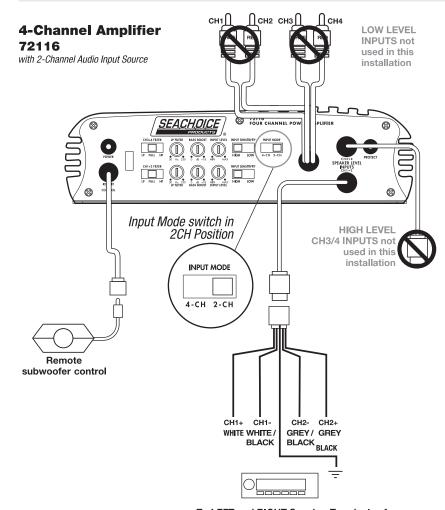
To LEFT and RIGHT Speaker Terminals of head unit or signal processor
