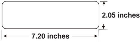
Insert mounting sleeve into the dashboard and bend the mounting tabs out with a screwdriver.
