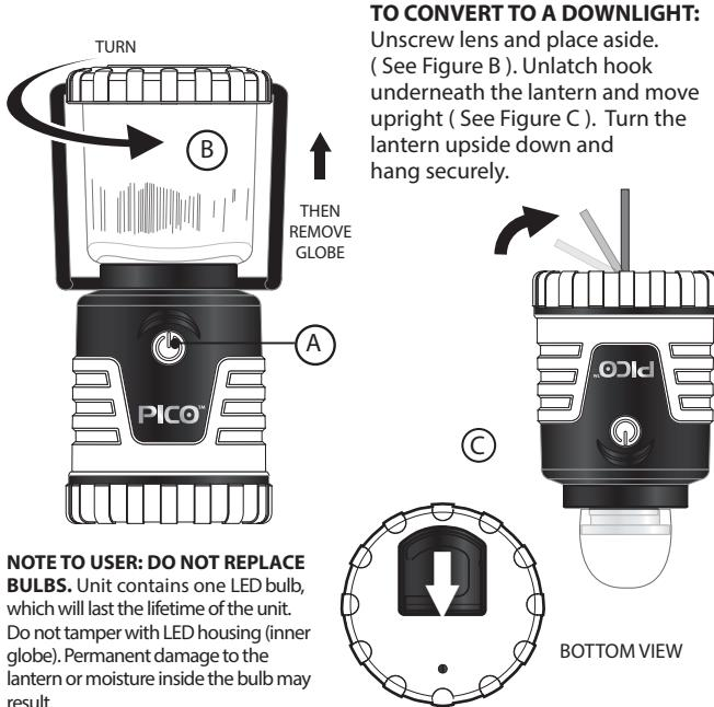
**NOTE TO USER: DO NOT REPLACE BULBS.** Unit contains one LED bulb, which will last the lifetime of the unit. Do not tamper with LED housing (inner globe). Permanent damage to the lantern or moisture inside the bulb may result.
