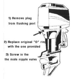
4) Attach female quick connect coupler to hose & flush
