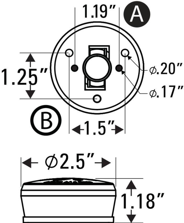
Twist-lock base for easy installation and hidden fasteners
