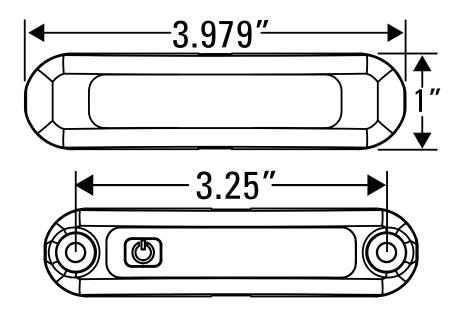
Hidden fasteners for a clean appearance 2 Mounting screws hidden behind the cover
