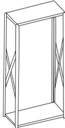
5. Flip unit so shelving is horizontal on floor or table. Bolt the second set of end frames to the unit creating a box.
