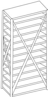
9. Stand the unit up and bolt a pair of long back braces together to form an "X".
