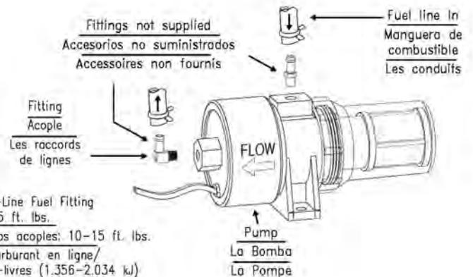
Note: Torque In-Line Fuel Fitting to 10-15 ft. lbs.
